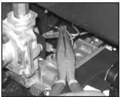
Figure 32: Remove Jumper From Thermocouple.
